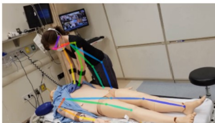
Fig 1: Still image taken from video data with OpenPose generated data overlain to create a skeletal representation of the patient and EMT. Video data is mixed with sensors worn by the EMT to determine the clinical procedure.
